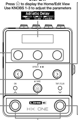
Press and release both the ON and TAP switches to display the Preset List
